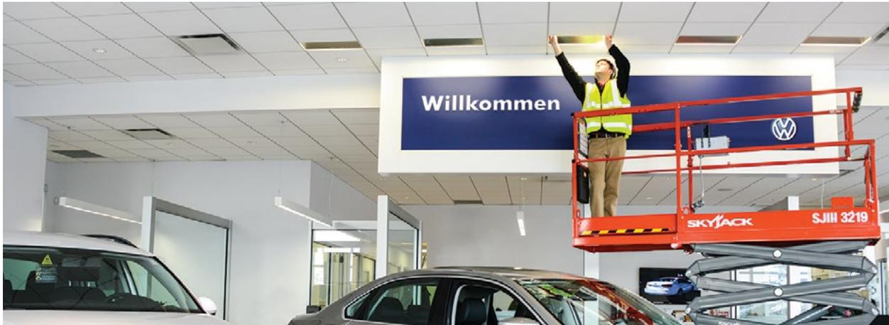
With the incorporation of a Motor Controller to the Skyjack Vertical Mast and S.JIII DC Electric Scissor Lifts, several things are different from the Hydraulic Proportional units. Operationally, the Hydraulic Proportional units control the speed of the functions by varying the flow of oil through the proportional valve. For the Motor Controlled units, the speed of the pump motor is varied to regulate the oil flow.
