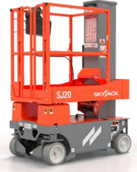
Robust all steel platform which incorporates a manually operated traversing deck feature which provides 16in of up-and-over capability. This can be released with a simple to use foot pedal, which and can be locked in various positions.
