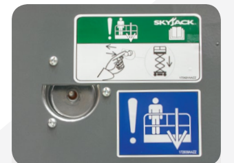
E-LOWERING Single location emergency lowering toggle switch integrated in hydraulic swing out tray. No more access rod required.
