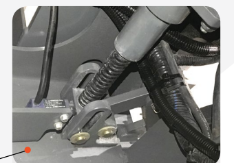
POTHOLE PROTECTION Directly mounted to the chassis with a simplified mechanical design. Ground clearance has been improved by up to 45%.
