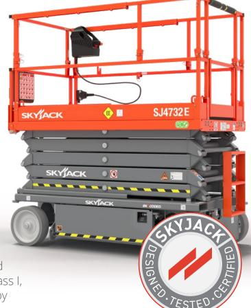
Classification: Skyjack scissor lifts equipped with "EE" Rating Package can be used in Class I, Division II, Group D locations as specified by the NFPA 505 Fire Safety Standard.
